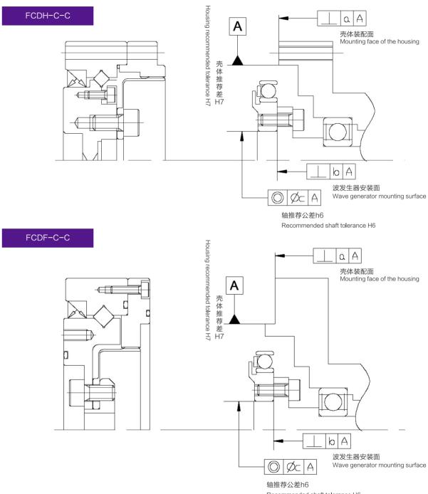
Recommended shaft tolerance H6
